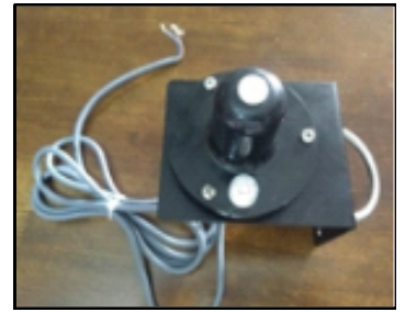
Silicon based Irradiation Sensor
